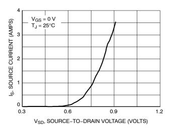
Figure 10. Diode Forward Voltage versus Current
