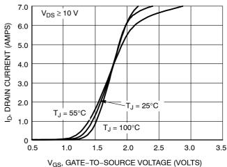
Figure 2. Transfer Characteristics
