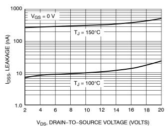
Figure 6. Drain-to-Source Leakage Current versus Voltage
