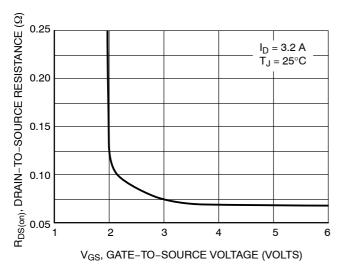
Figure 3. On-Resistance versus Gate-to-Source Voltage
