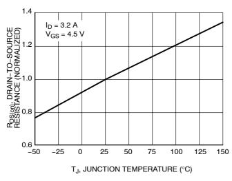
Figure 5. On–Resistance Variation with Temperature
